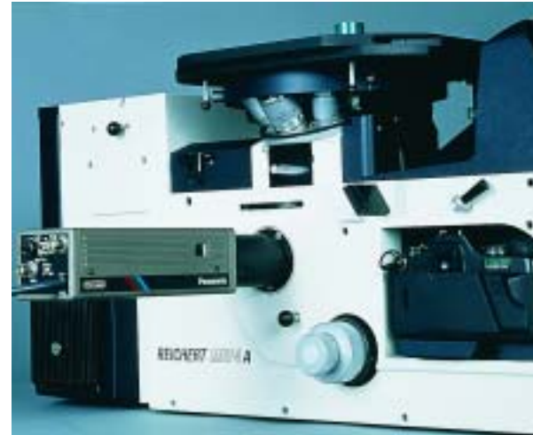
TV-widefield exit, factor p=0.66x Various cameras may be connected in conjunction with different adapters
