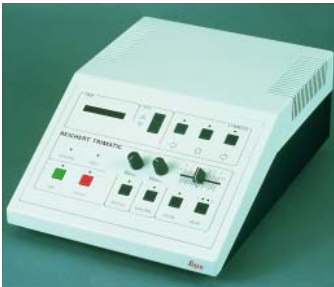
Control unit for automatic twin camera system
