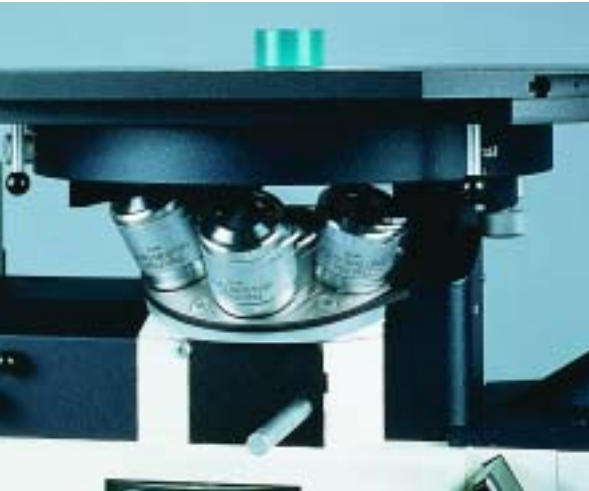
Motorized sextuple turret carrying the high quality lenses
